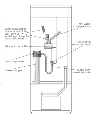
available, the water must be supplied through an ion exchanger connected in series. Connect water intake of the ion exchanger with the furnished hose to a tap water supply according to DVGW (avoiding reflux) which can be shut-off.
