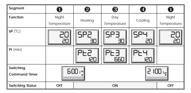
The moment for the command 1 OFF is calculated: **time end + time start + Pt2 + Pt3 + Pt4**, **i. e. our example**: 6.00 h + 120 min + 660 min + 120 min = 6.00 h + 15 h (3 h p.m.) = 21.00 h (9 h p.m.)
