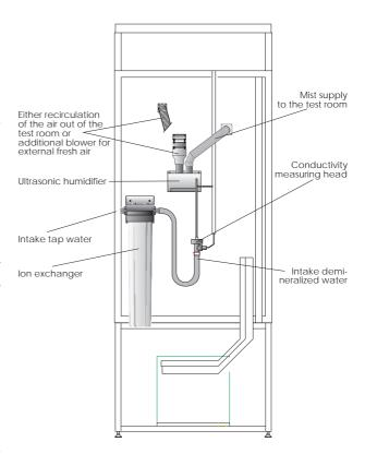
intake of the ion exchanger with the furnished hose to a tap water supply according to DVGW (avoiding reflux) which can be shut-off.
