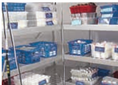
Stability test of drugs according to the ICH Guideline in the climatic chamber.
