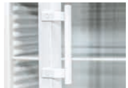
Free view on the specimen is ensured by an optional glazed door.
