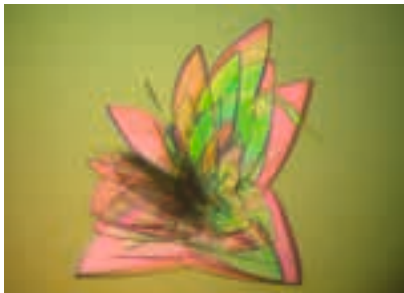
Protein crystals are very fragile: Freedom from vibration is a requirement for formation of these crystals.
